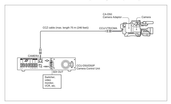
Use the procedure described on the next page to change the cabling in the SDI unit of this unit to SDI mode, and turn digital transmission on with the system setting switches.
