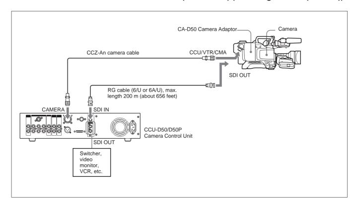
Check that the cabling in the SDI unit of this unit is set to VBS mode, and that digital transmission is turned off with the system setting switches. (See step 3 and 7 in "Connections for transmission over CCZ cable" on page 11.)
