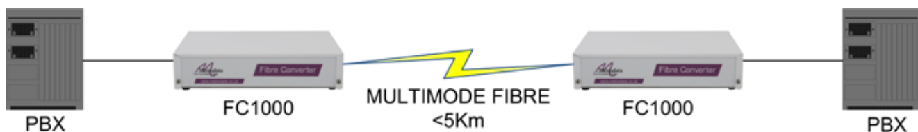
PBX to PBX extension over multimode fibre
