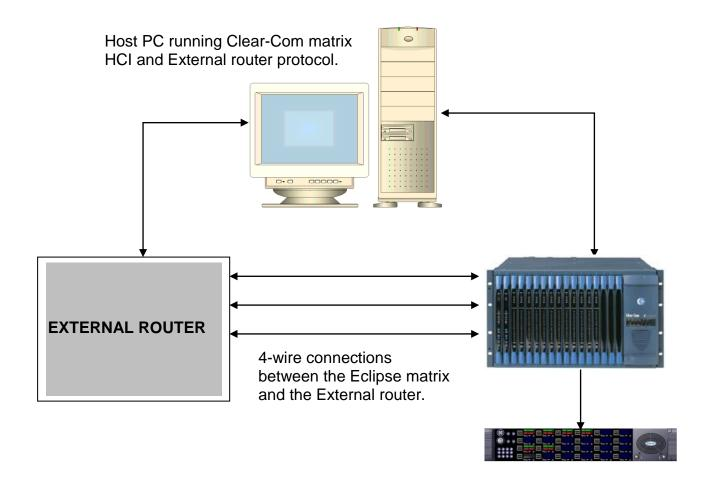
The Host PC receives routing information from the external router and translates this into the appropriate matrix HCI commands that are required to follow the external router actions.
