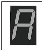
**Spectrum Friendly option:** Hold down the **CLR/BND** or **RESET REGISTRATION\*** button first then press and hold down the **REG** or **REGISTER BELTPAC\*** button till you see the letter "A" or "L" or "H".
