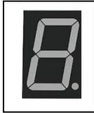
Powering on any DX base stations will produce on the LED display the number “8” for approximately 3 seconds followed by the following:
