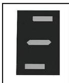
Three horizontal bars indicate the base is in secondary mode and has been linked with a primary base but that the primary is **no longer** on and not tracking with the secondary. It could take a few minutes for the secondary to recognize that the primary is not available.
