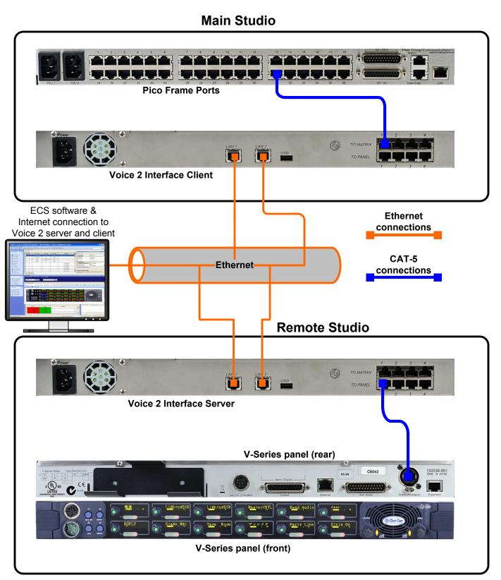
Connect the Eclipse frame panel port to the Voice 2 "To Matrix" port. Connect the V-Series panel "Matrix Comms" RJ-45 connector to the Voice 2 interface "To Panel" port. Both Voice 2 units need to have ethernet connectivity to each other (one Voice unit is the Server, the other is configured as the Client. Using the LAN 2 connectors access the Voice 2 software GUI to program the port properties. When properly configured the V-series panel will connect to the "remote" Eclipse frame.
