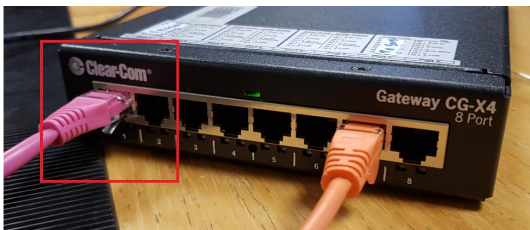
Fig 3 – MVX CAT5 connection to Gateway; these connections must match with how the Gateway ports have been configured ie: MVX Tel-14 port 1 to Gateway port 1 etc . .
